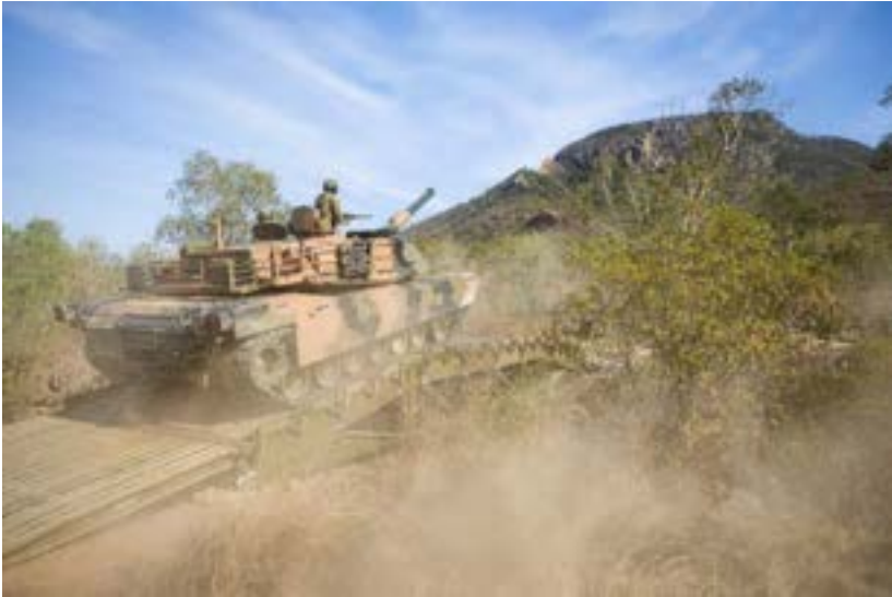
Figure 3.4: An M1A1 Abrams main battle tank crosses a medium girder bridge at Lavarack Barracks, Townsville
